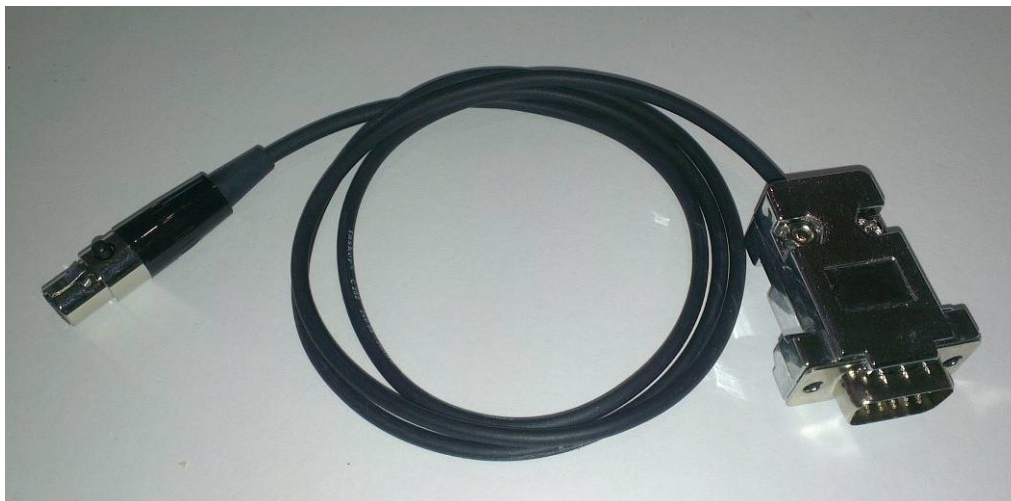
BMS-Charger communication cable (FES KOP601, FES KOP1001)
