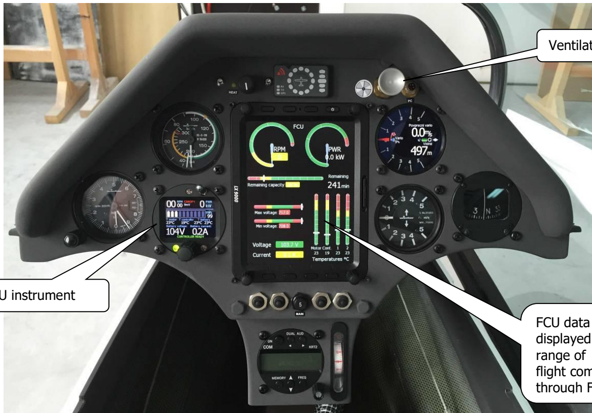
Suitable position for the FCU instrument on the panel of Ventus 2cxa FES
