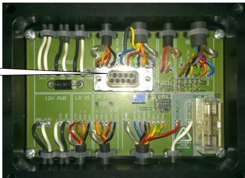
FCC (FES connecting circuit) with cover removed
